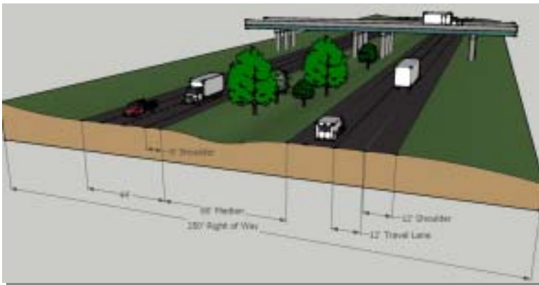
Picture 9: Roadway Classifications – Interstate
